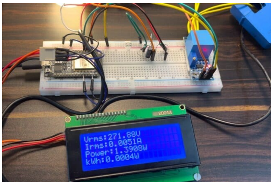
Fig. 3: Hardware implementation of the smart meter system
