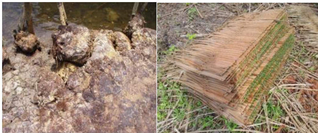
Figure 10: Photograph showing a mud dump used as infill for elevated mud foundations.
