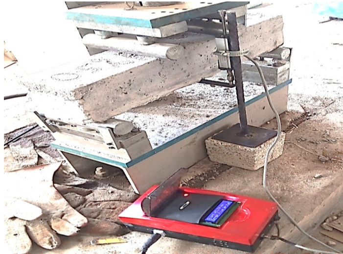
Plate II: Loading arrangement for testing load-deflection relationship.
