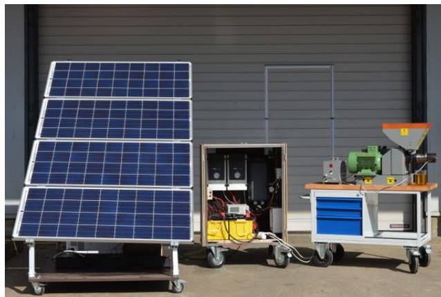
Figure 8: Sesame oil extraction solar energy system designed by the University of Hohenheim (Yadav et al., 2022)
