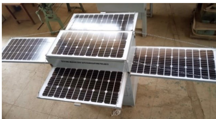
Figure 5: Foldable and mobile onsite power supply for rural communities designed by the Federal Polytechnic Nasarawa
